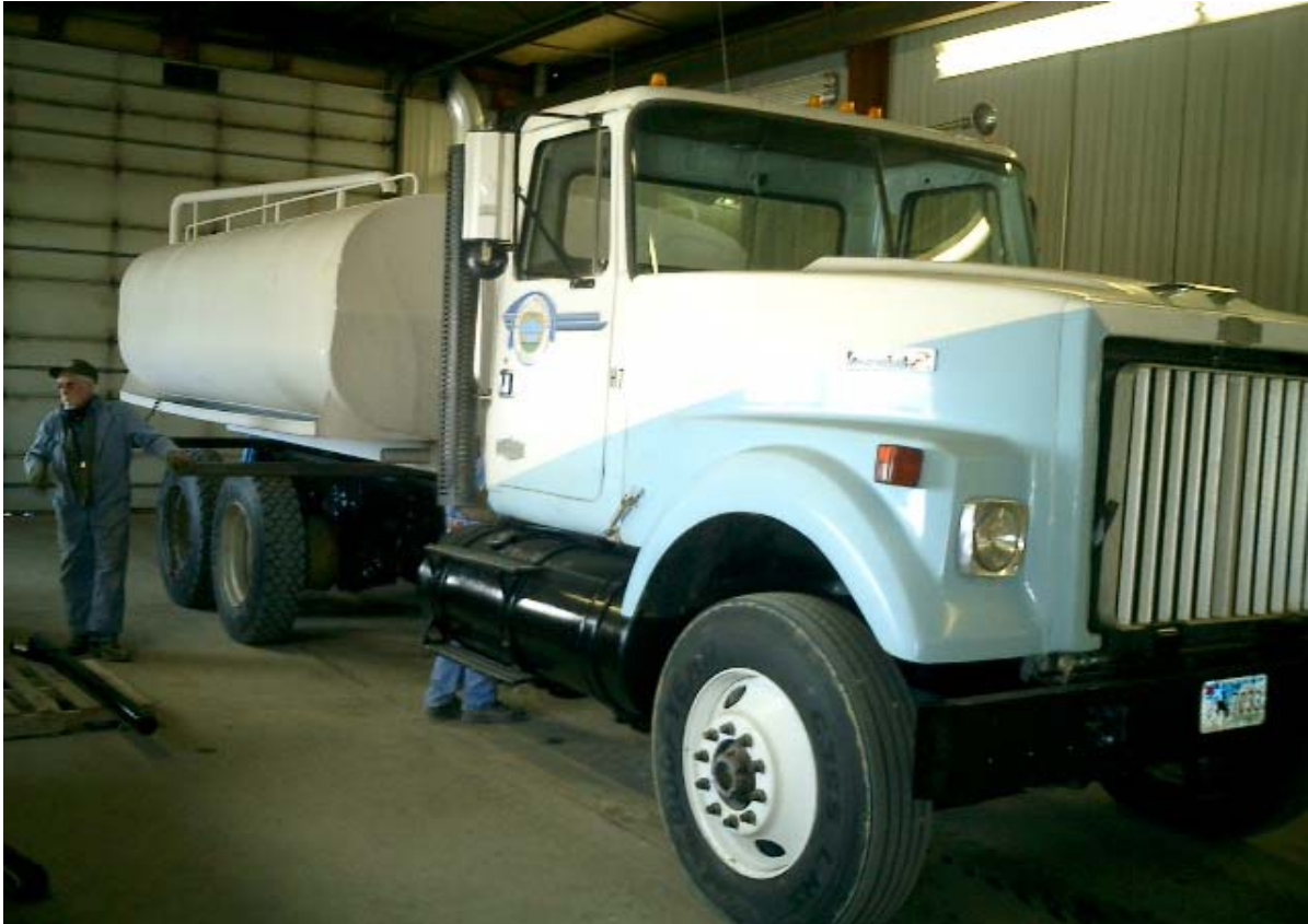
Figure 11. 1980 Autocar Dump Truck Converted to Water Truck
